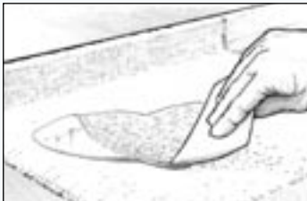
Figure 29 Spread the epoxy over the cloth surface with a plastic spreader.
