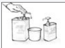
Figure 2 Dispense the correct proportions of resin and hardener.
