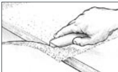
Figure 25 Trim excess cloth after the epoxy gels but before it cures hard.
