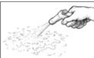
Figure 33 Rinse the surface with fresh water after sanding.
