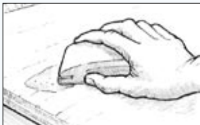
Figure 23 Sand cured fairing compound to desired contour.
